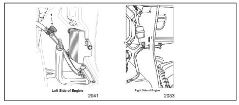
Figure 4-26 Fuel Shut Off Valves
